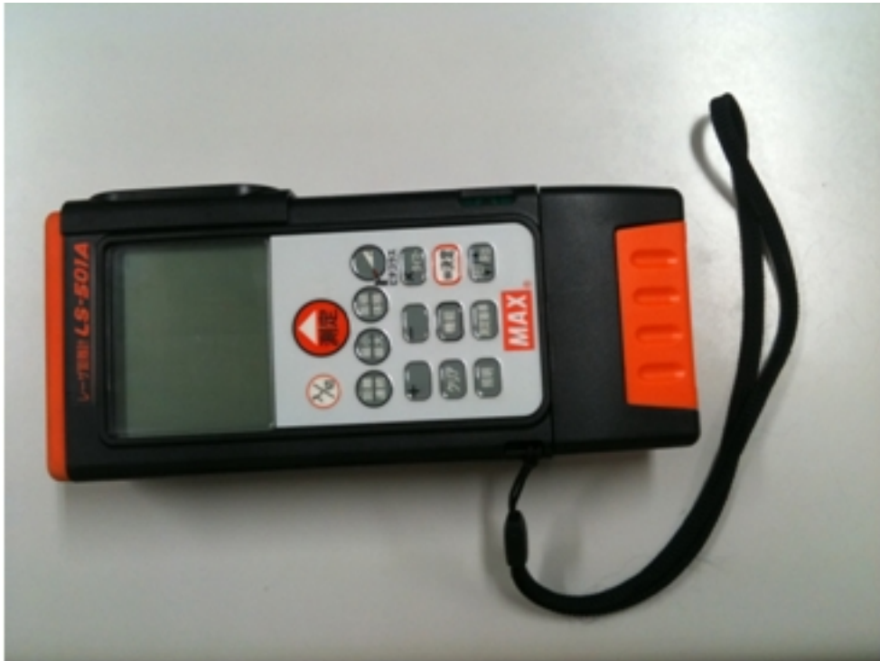
Figure 4.3.: Laser measurement equipment (LS-501A; MAX Co., Ltd.)
